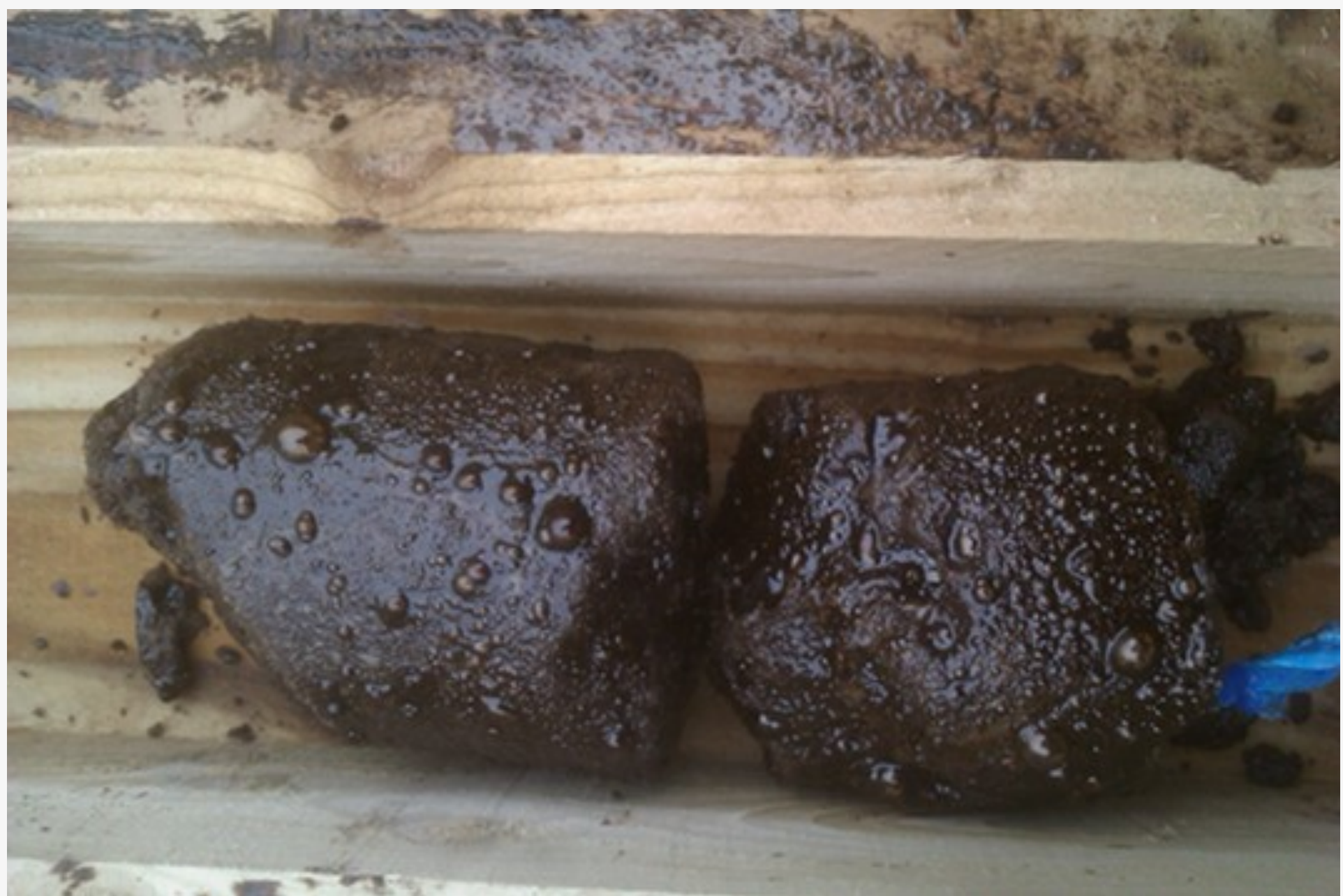
Oil-soaked Core Sample - Ormskirk Sandstone, Formby Oilfield
